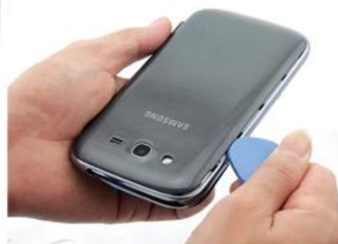
Paddles open shell external screen from the screen below double-sided adhesive peel
