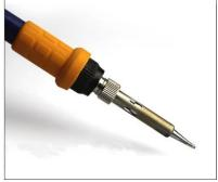
Clean the nozzle with solder sponge. Plating on the new tin layer, the soldering iron mouth can be clean as new.
