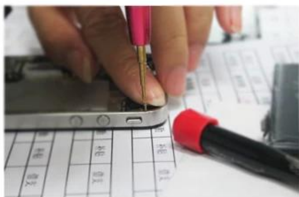
Screwdriver demolition internal screw
