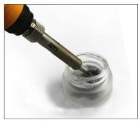
Let the welding nozzle and the solder regeneration grinding agent rub repeatedly.
