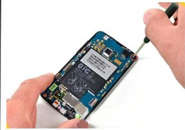
Screwdriver: demolition internal screw
