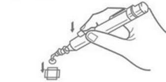
④ Put the IC on appointed place, press the button, the vacuum pen discharges air to let the IC fall off.
