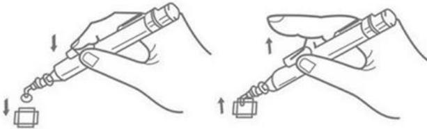
③ Press the button on the suction pen to discharge the air, then release the button to produce vacuum suction force to pick up IC.
