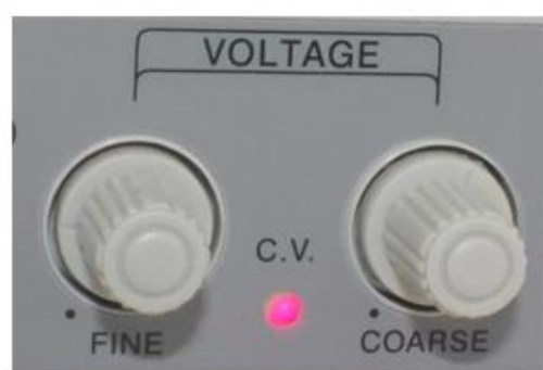
Voltage FINE / COARSE adjustment knob Regulators indicator
