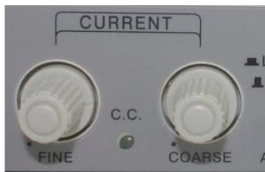
Current FINE / COARSE adjustment knob Steady flow indicator
