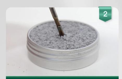
Let the soldering iron tip repeatedly rub against the repair paste
