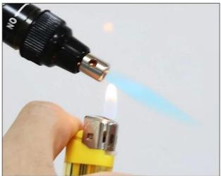
Install the flame head, can be used when spray guns
