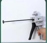
Install the plastic push rod into the glue gun (serrated side down)
