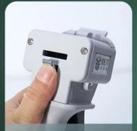
Push all the way up against the metal tab on the back of the glue gun
