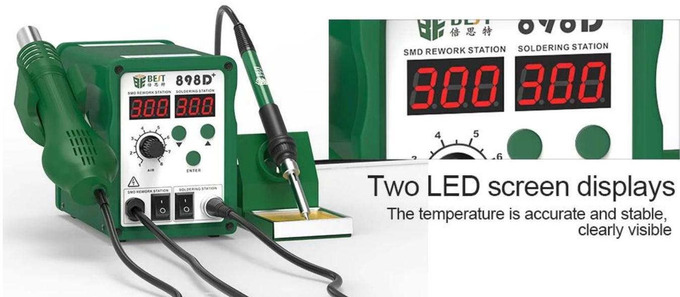
Imported ceramic heating core, the handle is made of high temperature resistant silicone wire.
