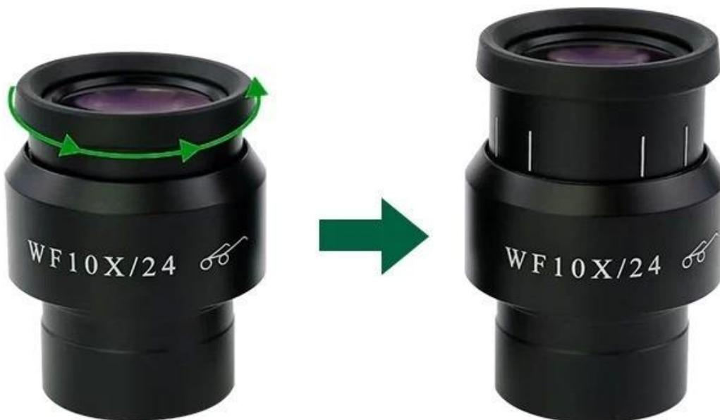
It can be adjusted according to the different visual acuity of the two eyes to achieve clear vision for both eyes
