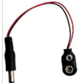
9V charging line
