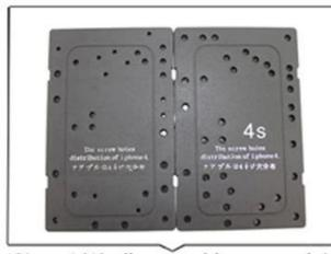
iPhone4/4S disassemble screw plate
