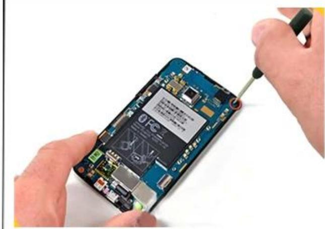
Screwdriver: demolition internal screw
