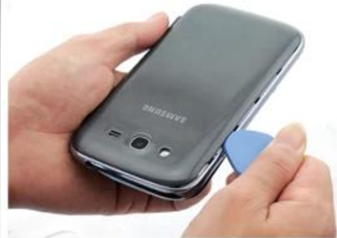
Paddles, stripped from the screen and the external screen below the double-sided tape to open the phone shell
