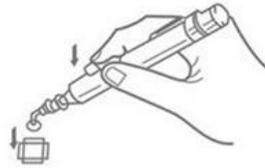
④ Put the IC on appointed place, press the button, the vacuum pen discharges air to let the IC fall off.
