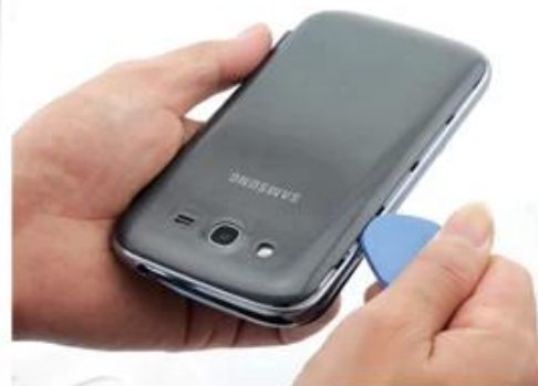
Paddles open shell external screen from the screen below double-sided adhesive peel
