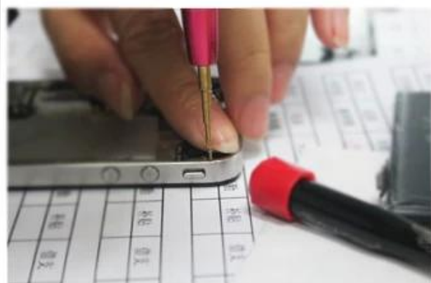
Screwdriver demolition internal screw
