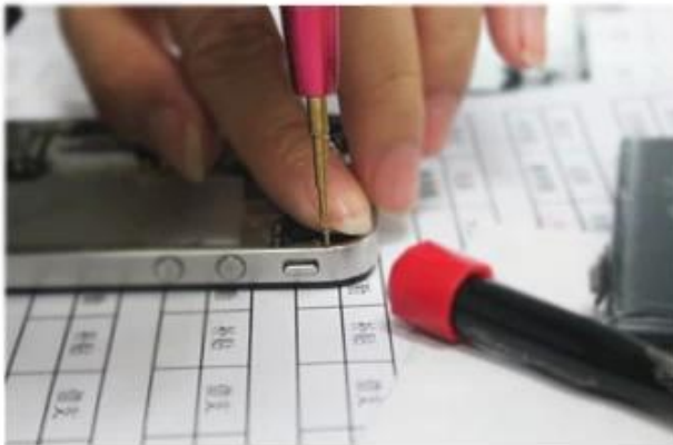
Screwdriver demolition internal screw
