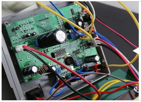
Integrated motherboard (reducing the number of multi-line connected together, performance has greatly improved in all aspects) Model and model unified motherboard (BST brand) Large transformer:
