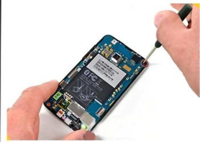
Screwdriver: demolition internal screw
