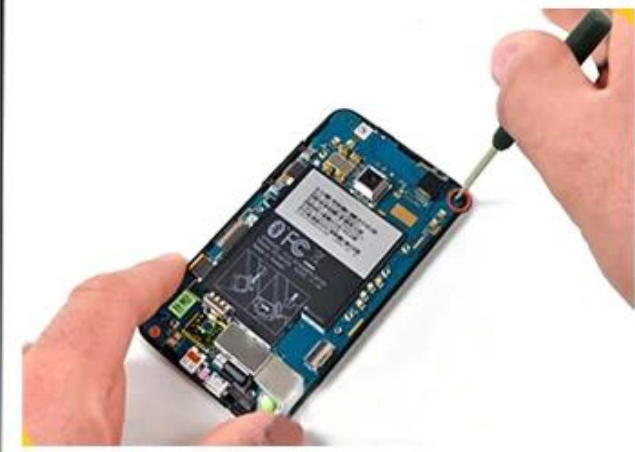
Screwdriver: demolition internal screw
