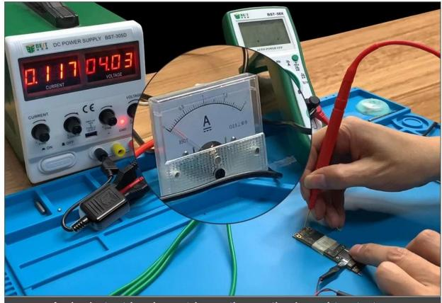
A single test lead can trigger the motherboard to start up
