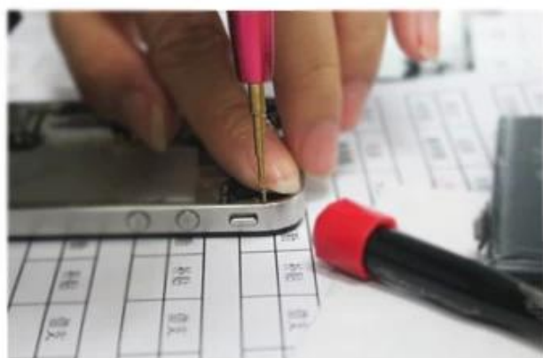
Screwdriver demolition internal screw
