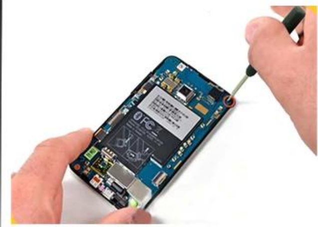
Screwdriver: demolition internal screw
