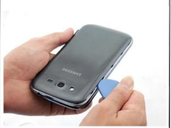
Paddles, stripped from the screen and the external screen below the double-sided tape to open the phone shell
