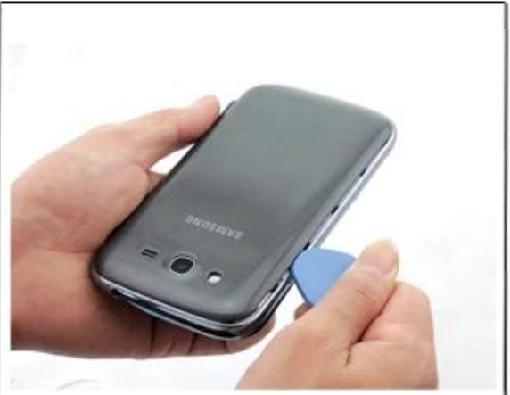
Paddles, stripped from the screen and the external screen below the double-sided tape to open the phone shell
