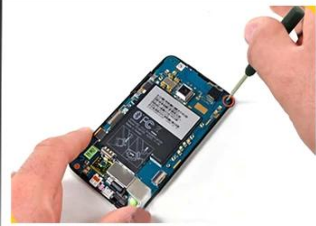
Screwdriver: demolition internal screw
