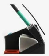
After a long period of inactivity, the tool will cool to room temperature.
