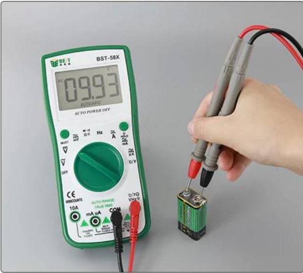
DC voltage measurement
